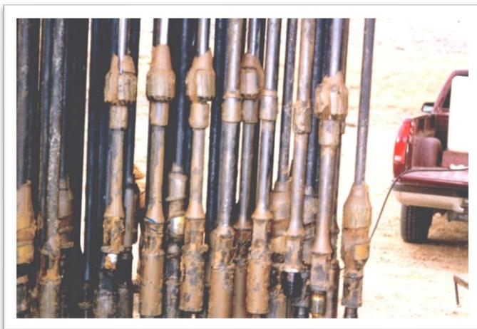
This picture is of rods which had been paraffined up and stuck in a 9,000 foot well in the Scott Field of Wyoming. A treatment of microbes was pored down the tubing and after two weeks operators were able to pull the rods. Note that almost all the paraffin was removed by the microbes during that time.
