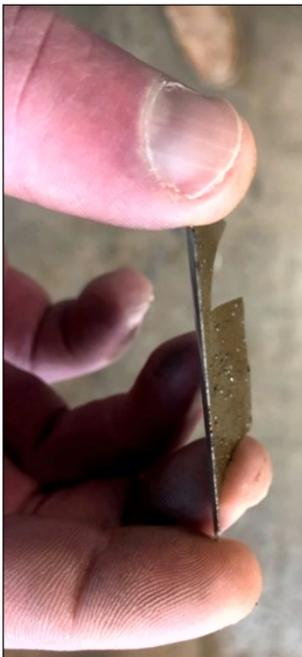
Metal with polysaccharide protective coating which is produced as a by-product of the microbial action
